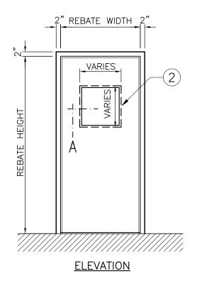
NOTE: — THE SIZES SHOWN IN THE ELEVATION REFER TO THE DOOR CUTOUT SIZE.
